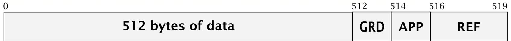
16-bit guard tag (CRC of 512-byte data portion)
