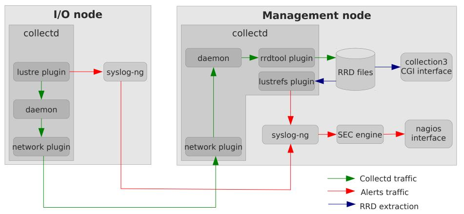
Collected data flow through collectd mechanism
