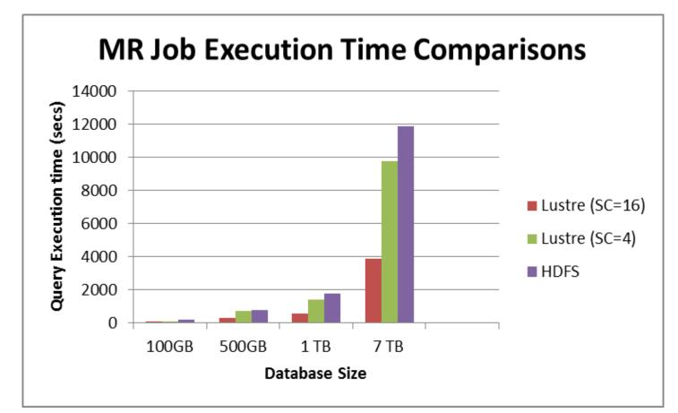
Intel® EE for Lustre\* delivered 3X HDFS for optimal SC settings
