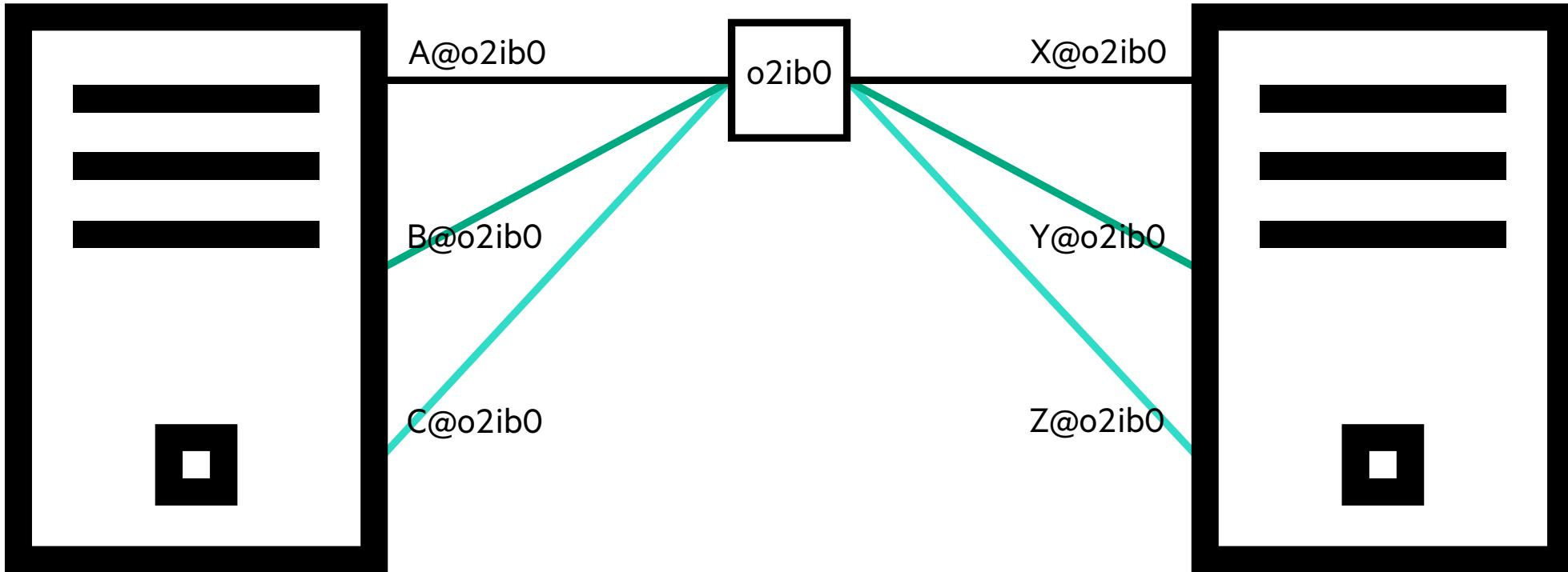
In Lustre 2.10, the LNet Multi-Rail feature allows for multiple interfaces in the same LNet network.
