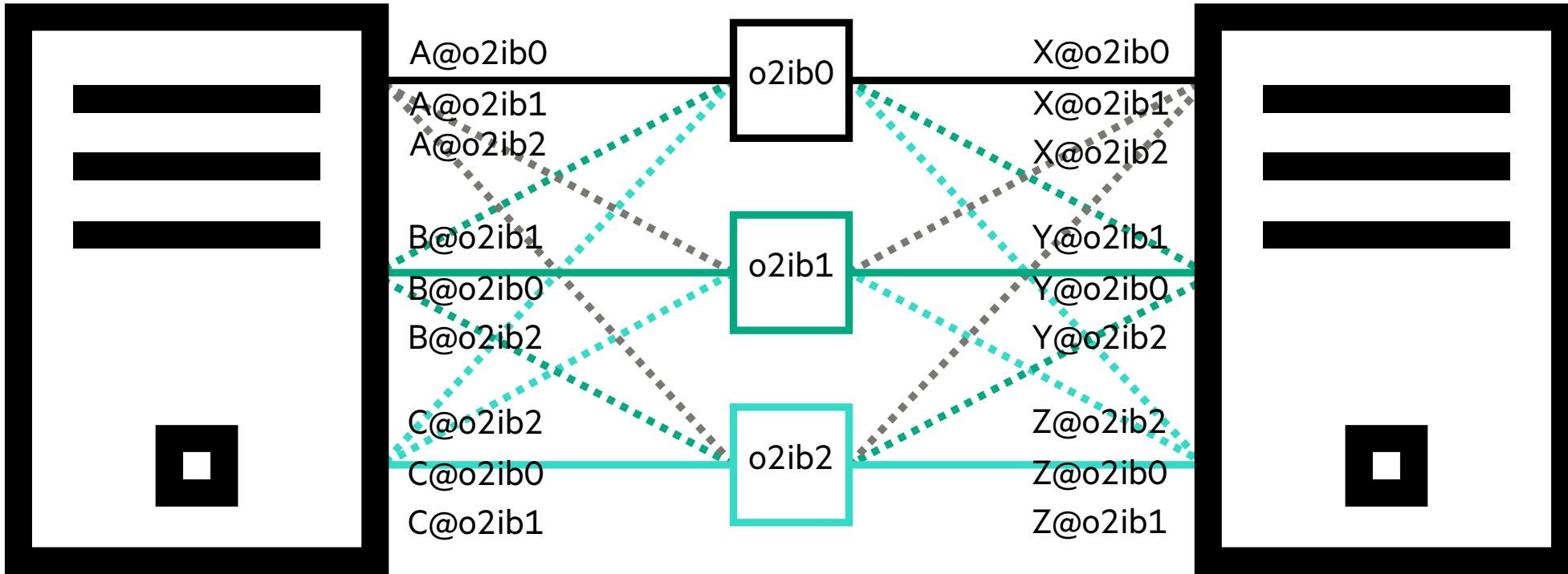
Aliasing used to facilitate communication to all networks.
