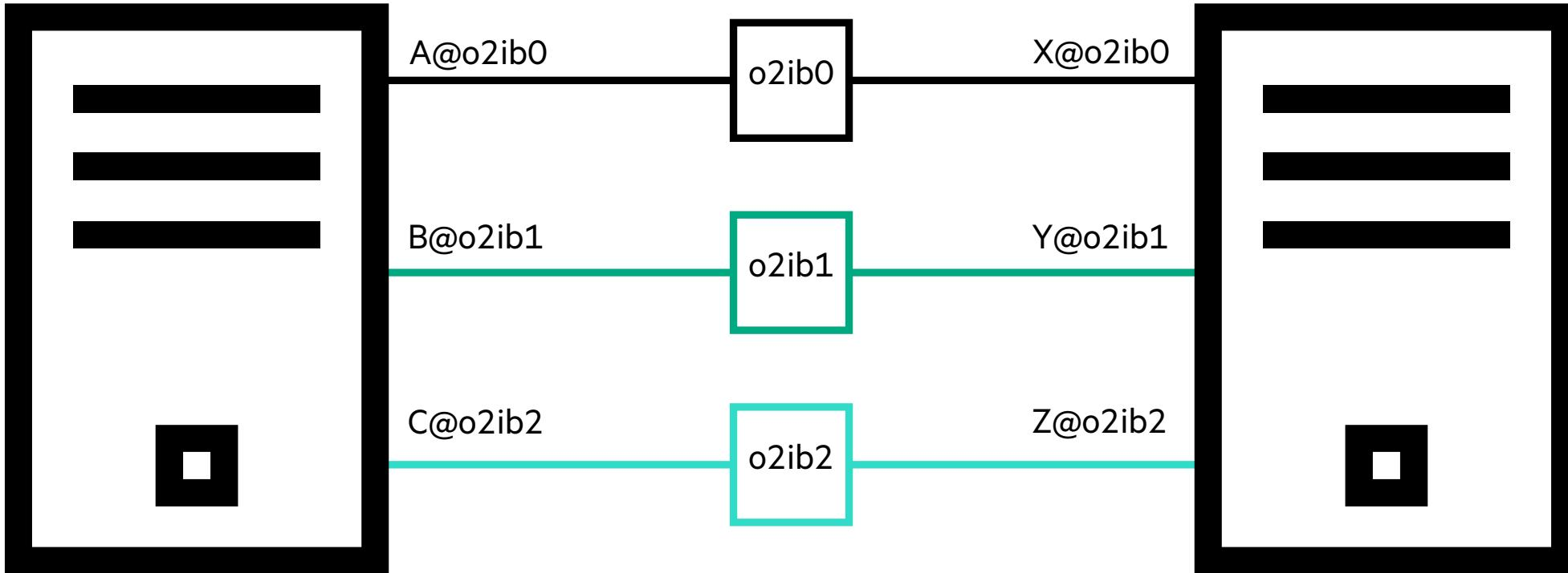
o2ib0 can't talk to o2ib1, or o2ib2
